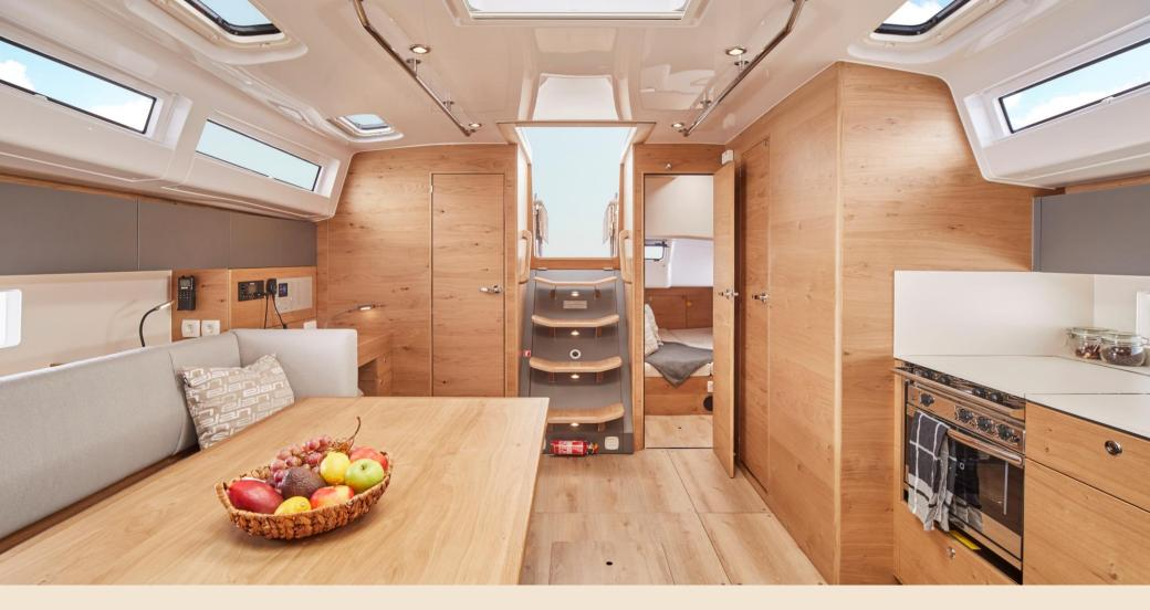
The interior is built with "rustic" oak veneer and marine-grade plywood, contrasted with modern gray-coloured storage cupboards.
